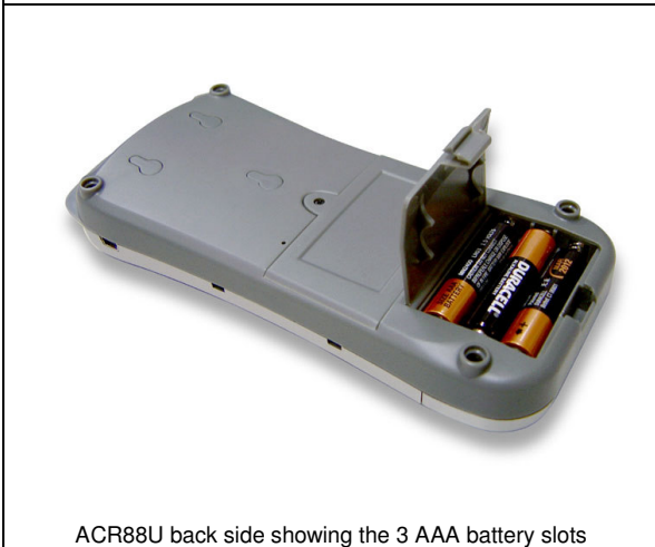
ACR88U back side showing the 3 AAA battery slots
